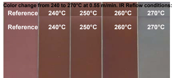
Color change from 240 to 270°C at 0.55 m/min. IR Reflow conditions:
