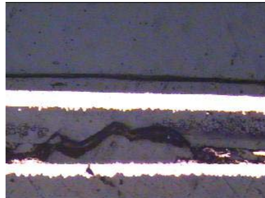
Picture 4. Failure within the dielectric itself
